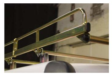
Make sure that everything is secure and don't forget to give your rack periodic spanner-checks over the next week or so just in case it needs any settling down on the roof and that's it; we suggest a nice cup of tea at this stage, and perhaps a biscuit.
